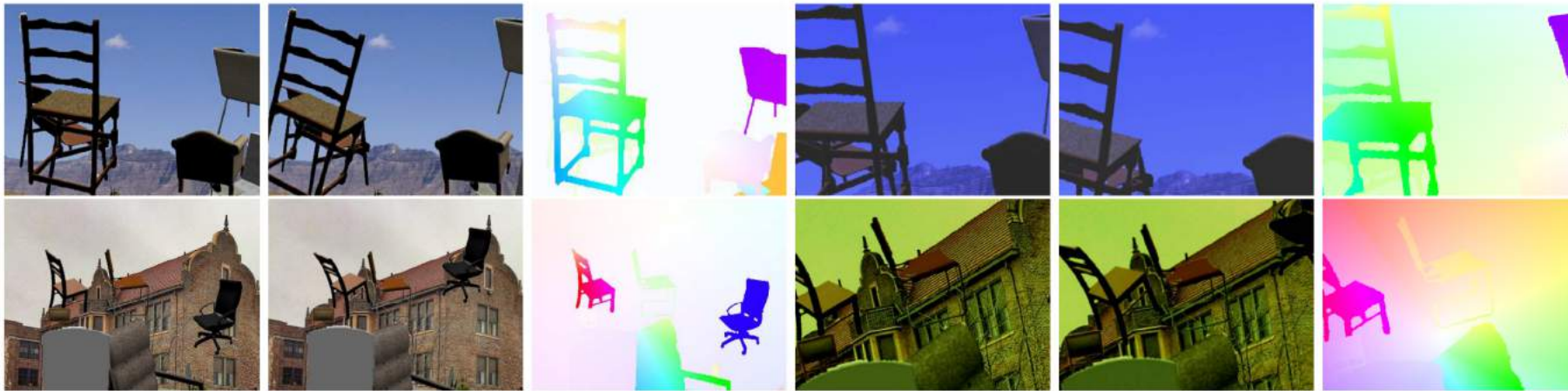
Figure 5. Flying Chairs. Generated image pair and color coded flow field (first three columns), augmented image pair and corresponding color coded flow field respectively (last three columns).
